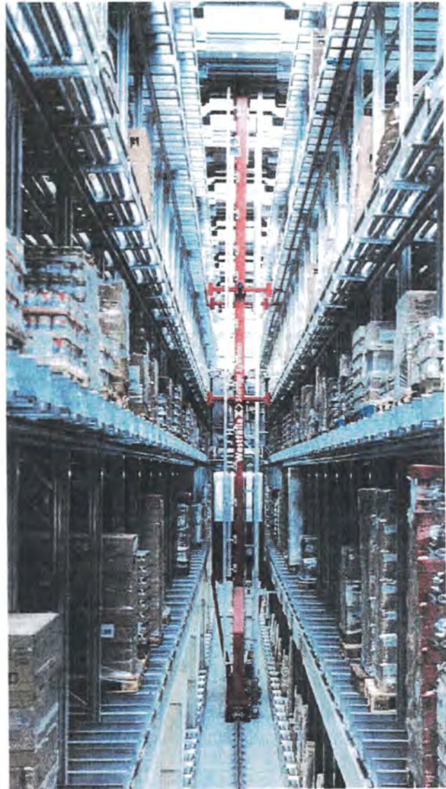
High Cube Warehouses utilize automated storage and retrieval systems (ASRS) to move and retrieve goods. Photo Courtesy of Westphalia Technologies, INC.
