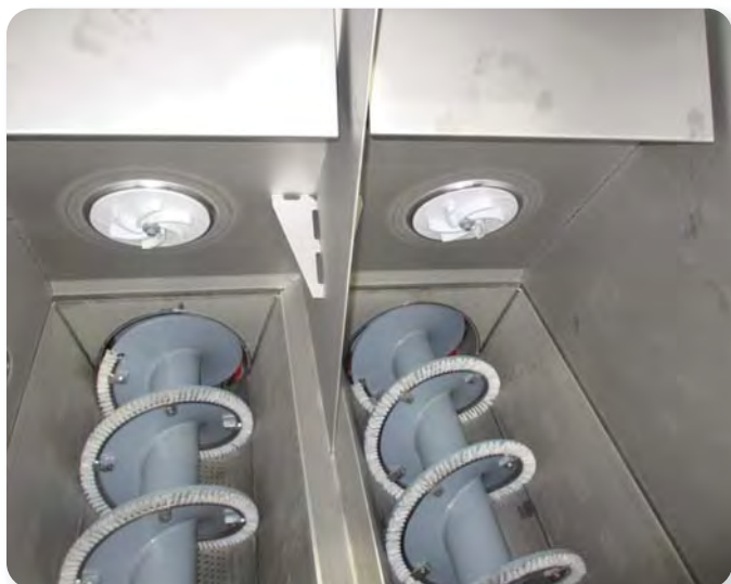
SPW 350-DM with optional impellers to increase washing function.
