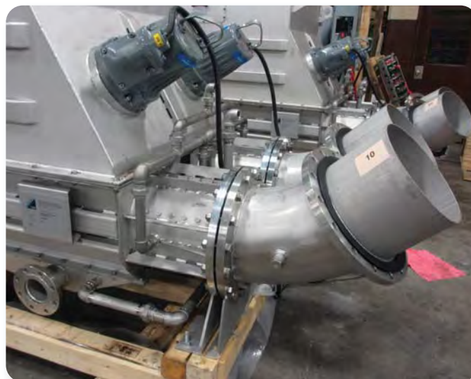
SPW 350-DM with optional impellers to increase washing function.
